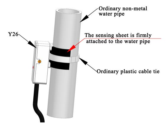
The height of the sensed liquid level is related to the sensitivity of the sensor. The higher the sensitivity, the lower the sensed liquid level
