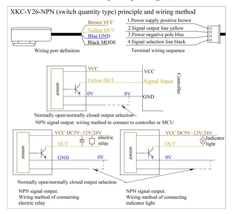
NPN output drives small electric relays (coil current ≤ 100mA) Product Applications:
